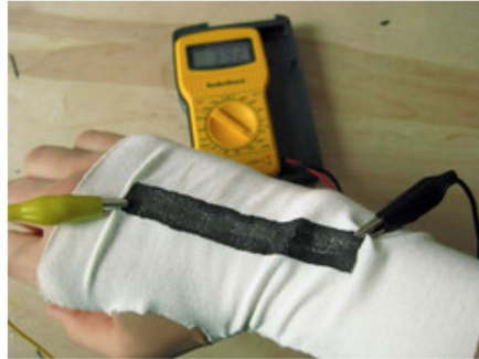
Constructed stretch sensors, by KOBAKANT DIY Wearable Technology Documentation
