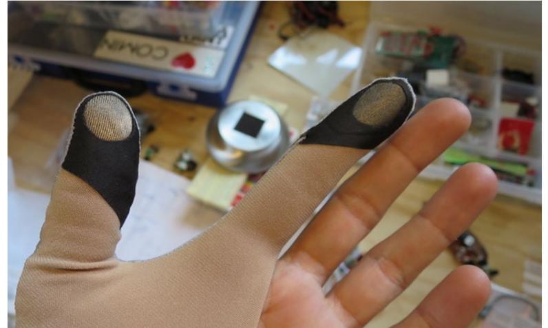
Fingertip contact switch, by KOBAKANT DIY Wearable Technology Documentation
