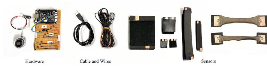
Fig. 1: The Toolkit: (a) USB cable for power; (b) audio cable for speaker; (c) speaker; (d) Bela embedded computer and breakout board; (e) sensors.
